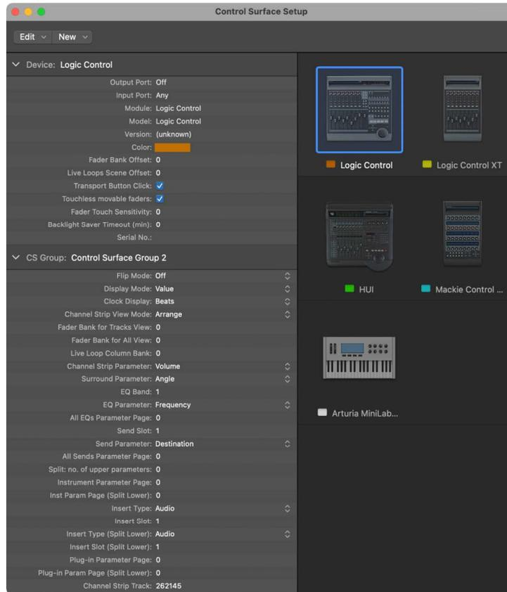
The top row, consisting of the Logic Control and Logic Control XT, forms a single control surface group with 16 channels. Logic Control controls channels 1 to 8 and the XT unit controls channels 9 to 16.
