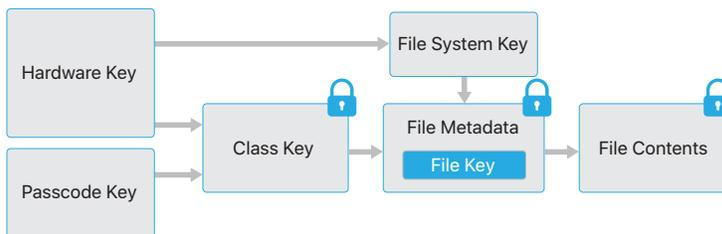
The contents of a file may be encrypted with one or more per-file (or per-extent) keys that are wrapped with a class key and stored in a file’s metadata, which in turn is encrypted with the file system key. The class key is protected with the hardware UID and, for some classes, the user’s passcode. This hierarchy provides both flexibility and performance. For example, changing a file’s class only requires rewrapping its per-file key, and a change of passcode just rewraps the class key.
