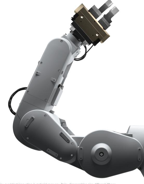
Meet Daisy, our latest innovation in material recovery. Daisy disassembles nine different iPhone models, so we can recover materials that traditional recyclers cannot—and at higher quality.
