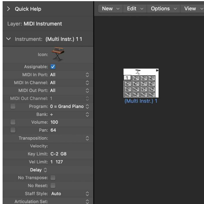
You generally use multi-instrument objects to address multi-timbral hardware synthesizers or samplers. A multi-timbral sound module is one that can receive on several MIDI channels at once, playing back a different sound on each channel simultaneously.
