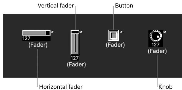
The auto style fader—the default style if you create a fader with a key command—changes styles as you alter its shape and size.
