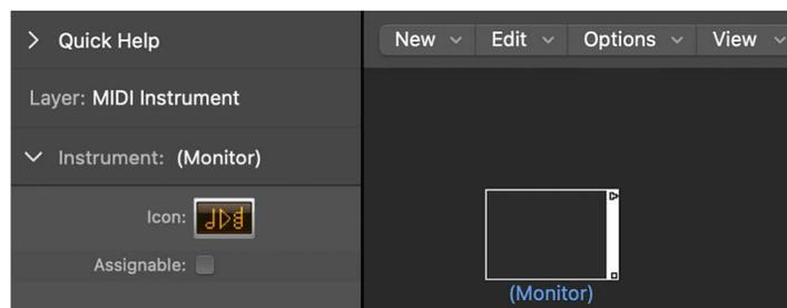
Monitors are useful as both testing and branching devices. When coupled with objects that have functionally different outputs (channel splitters and mapped instruments, for example), monitor objects can be used to attach more than one output cable to the same function.
