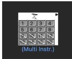
In the above image, subchannel 1 is selected, subchannels 1 to 8 are activated, and subchannels 9 to 16 have been removed from the Reassign Track shortcut menu.
