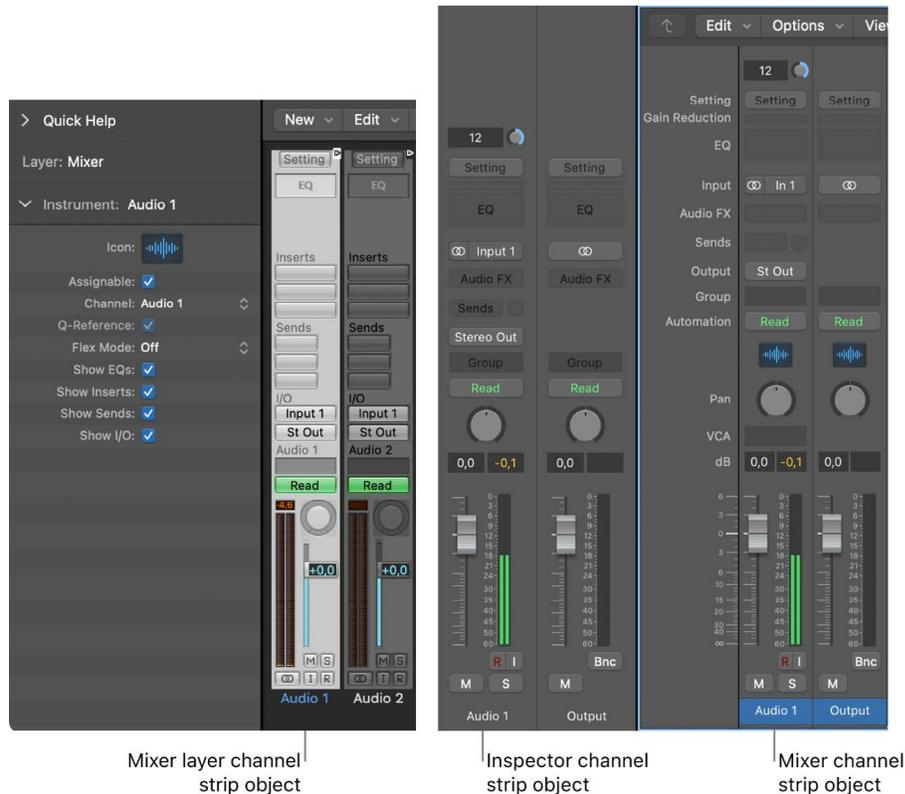
The audio and software instrument tracks you see in the main window are actually routed to channel strip objects on the Environment Mixer layer.
