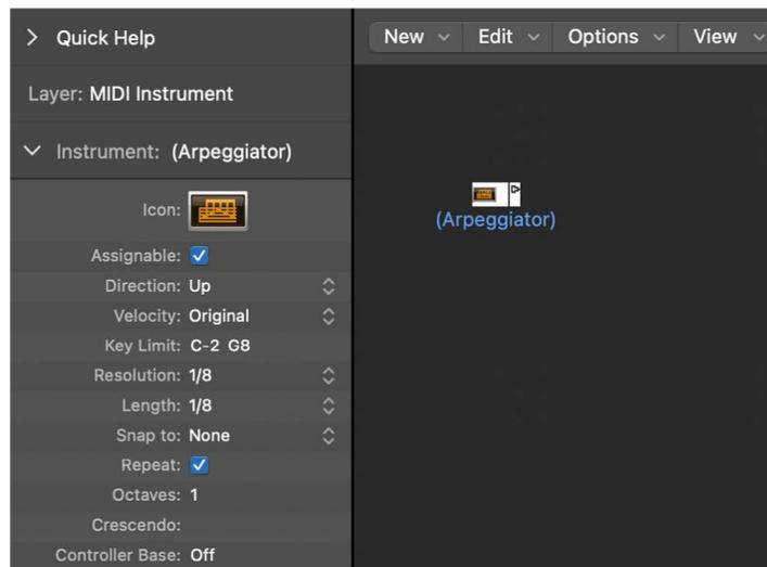
An arpeggiator features parameters for direction, velocity, speed (Resolution), note length, start quantize (Snap), repeats, octaves, and velocity offset (Crescendo). All parameters can be MIDI controlled in real time, which adds immensely to its versatility.
