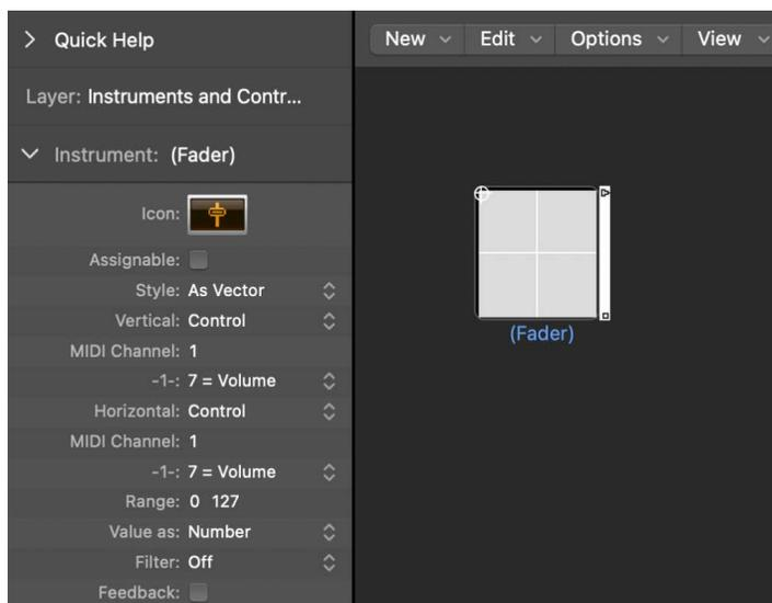
Most faders have Input and Output definitions, which determine the MIDI events sent by the fader (Output), and those it reacts to (Input). (See [Fader functions: range, value as.](#))
