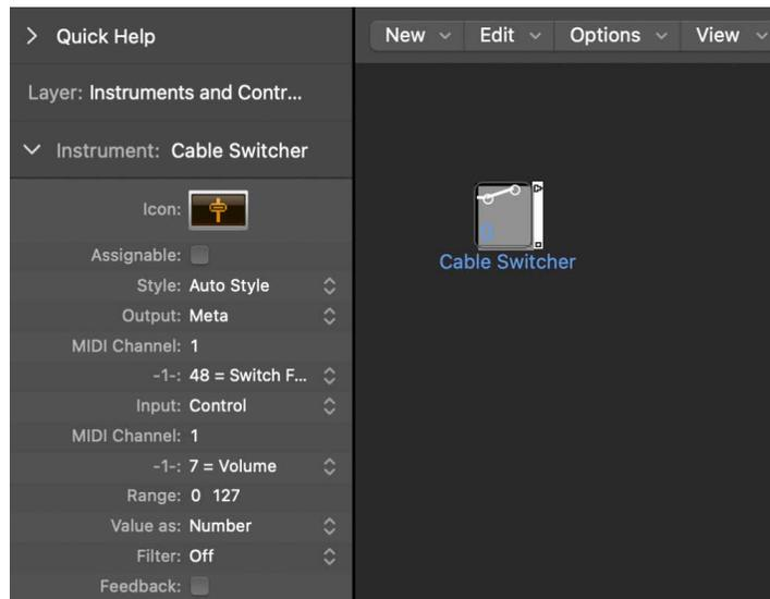
A cable switcher can be assigned to any fader style. It's practical to use the text fader style, as it allows you to label the switcher's various routes. Use Auto Style to actually display the switch routing, as shown above.
